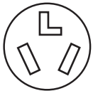
3-wire receptacle (10-30R)
