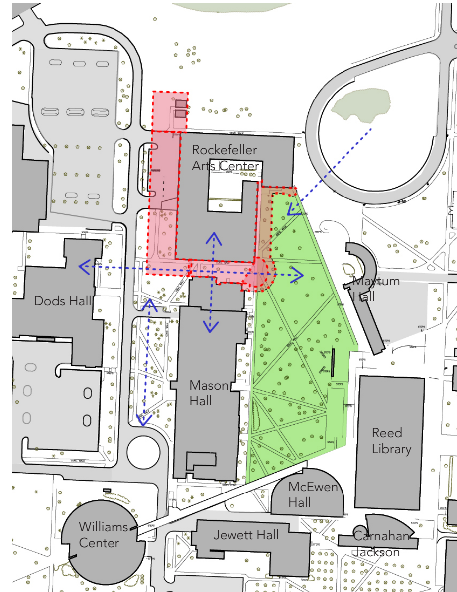
Conceptual diagram showing potential building additions to the Rockefeller Arts Center. Siting strategies include an extension of the Visual Arts wing, an infill atrium between King Concert and Mason Hall, and a new entry admission facing Symphony Circle.
